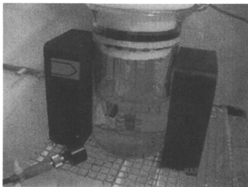
Figure 2. Cell 662 positioned in a magnetic field of 700 Gauss.
